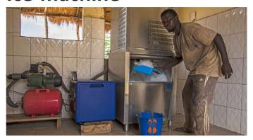
You need: Solarpanel, waterpump, Icemaking machine, water, capacitybuilding in solar technology and business.
